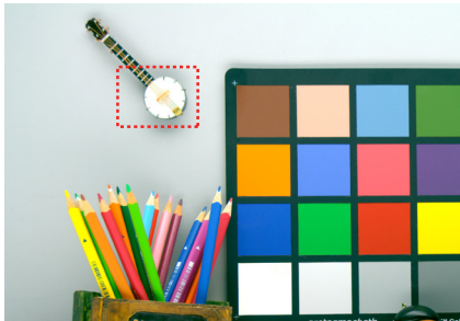
Figure 12: Properly exposed bright light scene, 2,430 lux daylight illuminant, 125ms, enabled by the LCG mode of Aptina's MT9H004 sensor with Aptina DR-Pix technology.
