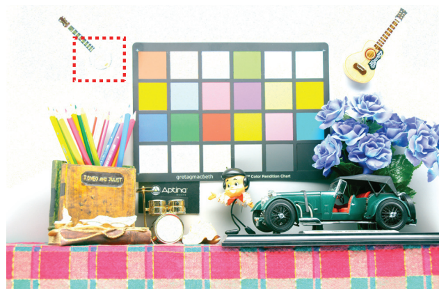
Figure 10: Overexposed scene using HCG in a 2,430 lux daylight illumination scene with 125 ms of exposure time.
